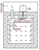
**Easy to clean and service.** Cleaning is easy due to the scratch-resistant, baked enamel exterior, 304 stainless steel interior, and smooth door surface. Servicing is easy due to convenient top access to the heater and fan.
