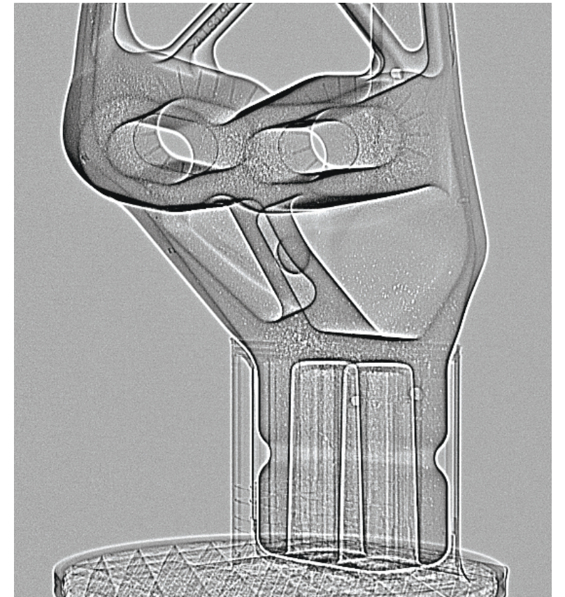
Side mirror X-ray image with optimized settings for manual 2D inspection.
