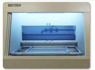
The GSR1290 is a single table standalone router machine specially designed to route (depanelize) large panels with PCB sizes of 910mm x 610mm into individual units. It is capable of speeds of up to 100mm/s and positioning speeds of 1000mm/s. The superior servo axis system provides a high acceleration/deceleration, reducing cycle time (increase in production output) and at the same time maintaining high accuracy cutting.
