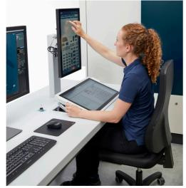
In the FF85 CT, software and hardware work hand in hand to make system operation as easy as possible. The clean layout of the operator desk with tiltable touchscreens allows users to stay focused on the inspection task. The height of the desk can be adjusted, facilitating operation from a sitting or standing position. Healthmonitor and push messages keep the user informed about system status and inspection progress at all times.
