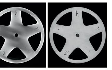
Eliminating unwanted gray-value gradients: Cone-beam CT without (left) and with Beam Hardening Correction (right).
