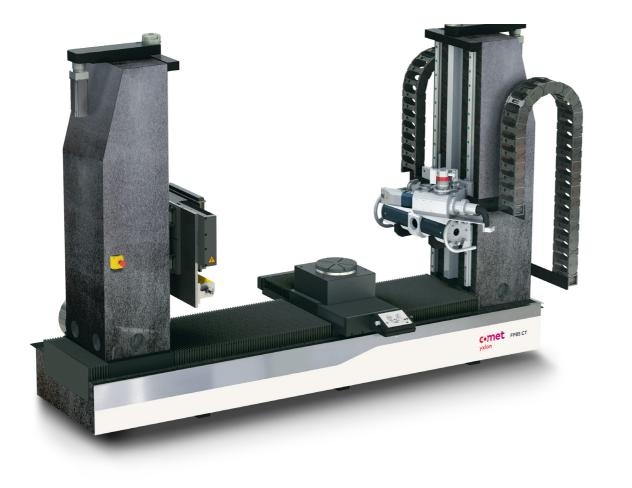
Small parts, large parts, dense materials - with its possible combination of two X-ray tubes, a spacious flat-panel detector and/or the CTScan 3 line detector, the FF85 CT is up for almost everything. Seamless switches between 2D radioscopy, 3D cone-beam, and fan-beam CT provide outstanding flexibility and allow for individual inspection processes.
