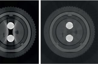
Reducing interferences: Cone-beam CT without (left) and with Metal Artifact Reduction (right).
