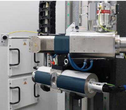
You can switch between the different tubes in one CT sequence.
