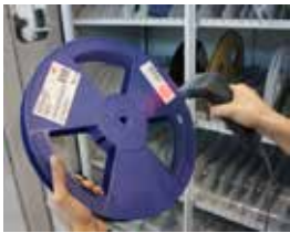
Read barcode for insertion and extraction of components
