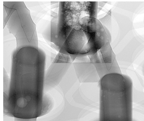
THT with voiding
