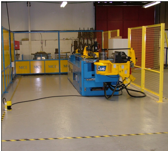
CNC Tube Bending —Up to 65mm Round complete with 'Push Bending'.
