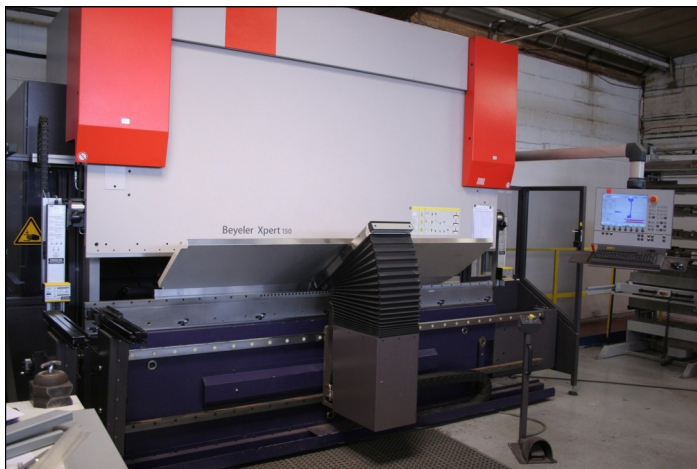
CNC Brake Presses —We have 4 in total, up to 3m and 8 axis.
