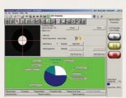
This innovative system utilizes texture-based image acquisition algorithms and a digital camera system with telecentric lenses to support the accurate identification of paste deposit defects.
