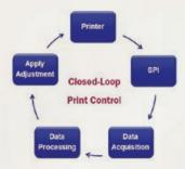
SPI Print Optimizer brings your Solder Paste Inspection (SPI) machine into communication with your MPM printer through a specially-developed common interface. When the SPI machine 'sees' X, Y and theta offset problems
