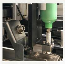
Temperature monitoring ensures proper paste viscosity to avoid bridging and voiding. MPM patent-pending paste temperature monitor allows paste to be measured in the cartridge or on the stencil.
