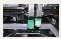
Dispense for standard cartridges or choose the new patent-pending jar dispenser. Paste is released in precise, measured amounts across the stencil in a
