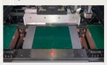
reduced distance on input conveyor by pre-loading the board during the print process results in reduced transfer times and improved cycle time.
