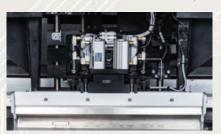
provides squeegee force, and a unique algorithm calibrates out non-linearity, maintaining the set pressure across the entire board surface.
